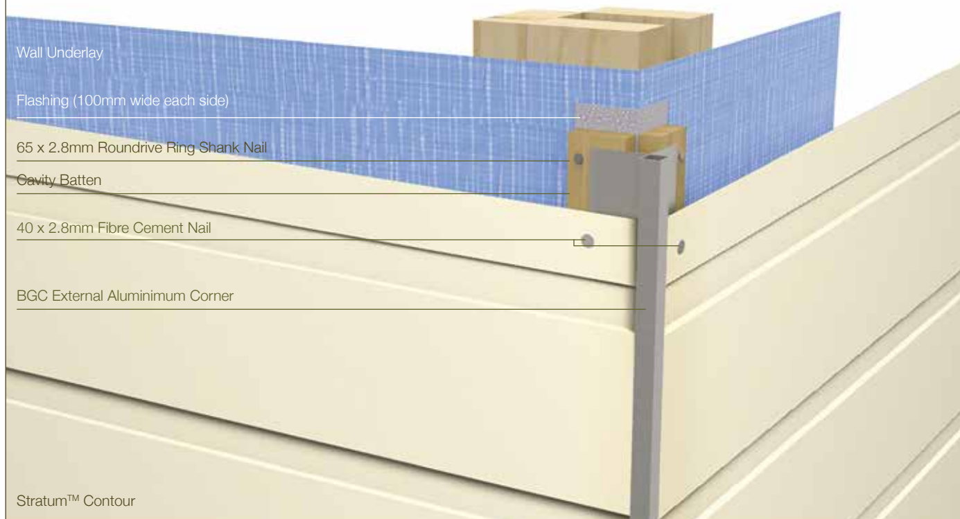
FIGURE 23 STRATUM™ CONTOUR - ALUMINIUM BOX CORNER
